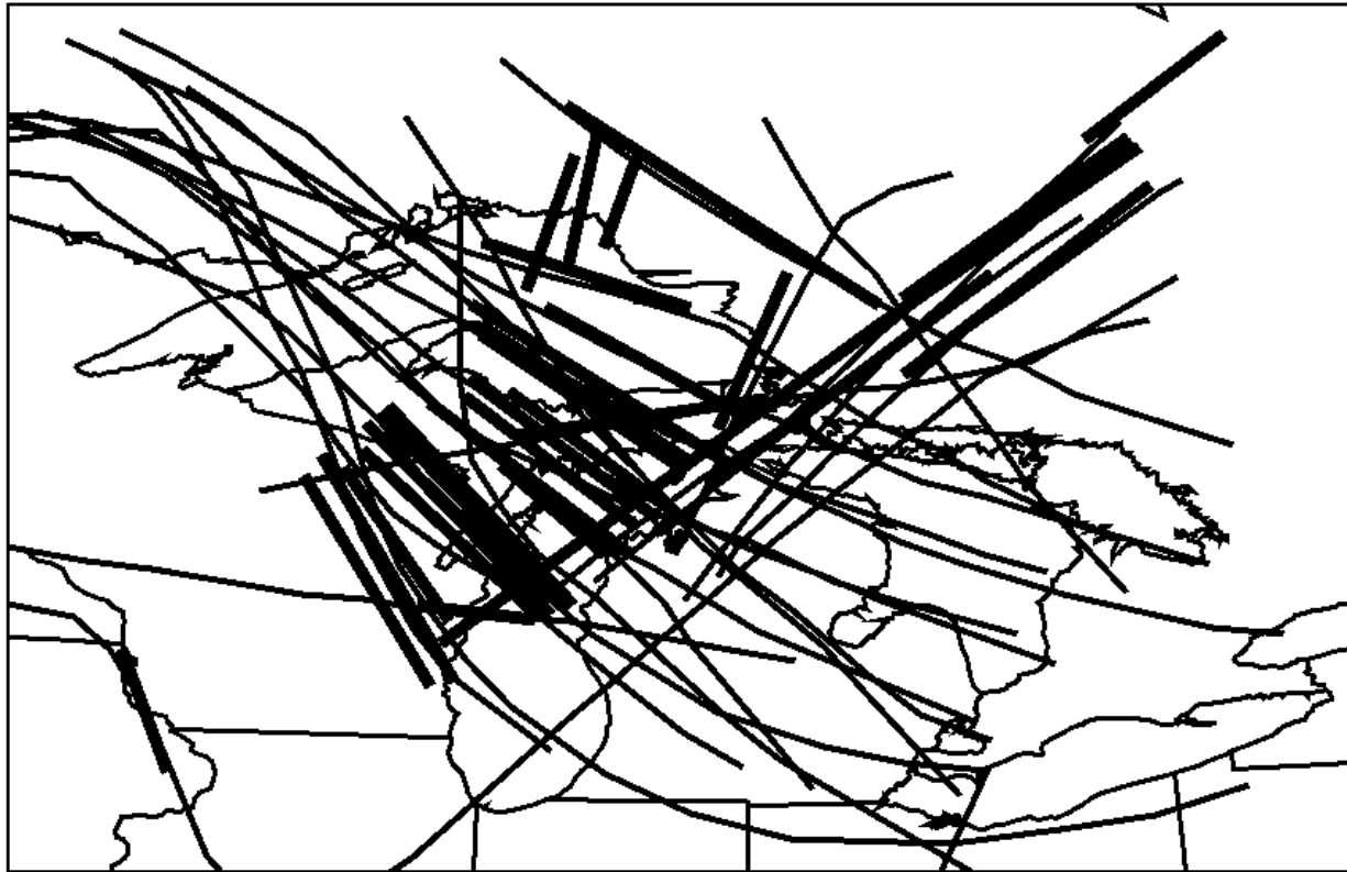
FIG. 10. Contrails visually identified in GOES-8 imagery (thick lines) matched with the nearest flight tracks of commercial aircraft from FT (thin lines) at 1745 UTC 9 Oct 2000. Flight tracks from earlier times were advected to the present time using the RUC horizontal winds at the level corresponding to the flight track altitude.
